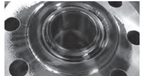
Penetrant testing is one of many possible NDT's for welds.
