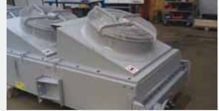
Transformer oil cooler with angled fan sections for efficient and directed evacuation of hot exhaust air to avoid re-circulation.
