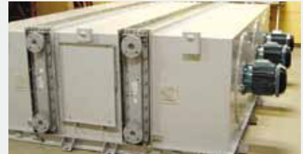
Hood installation. Complete cooler unit customized to fit client machine.
