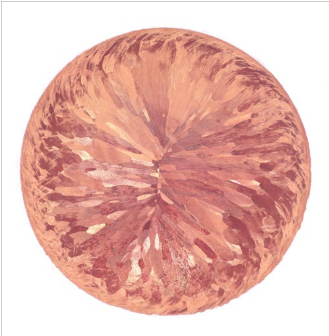
Figure 1. Luvata’s anode balls contain large cast grains.
